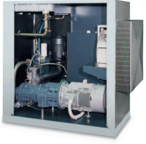
High-efficiency, low load-loss, 2 micron pleated **intake filter** with cyclonic pre-filter; the filter prevents damaging particles from entering the air and oil circuits, achieves improved oil efficiency and prolongs the life of the air/oil separator element and oil filter.
