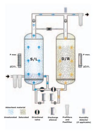
The next cycle starts with the inversion process. The moist compressed air passes through the regenerated pipe  $^{\rm (S/L)}$ , while the moist pipe  $^{\rm (D/R)}$  begins its own regeneration.
