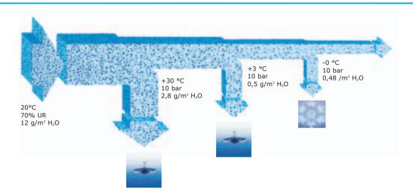
The cooling process does not allow the temperature to fall below 0°C (solidification of water). However, specific applications or particular ambient conditions require dew point temperatures of below 0°C.
