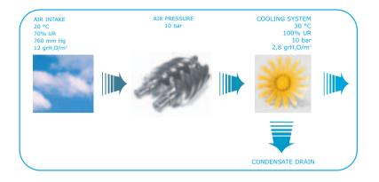
A compressor that operates in an ambient temperature of 20°C and 70% relative humidity takes in 12g of water for every Nm<sup>3</sup> of air.
